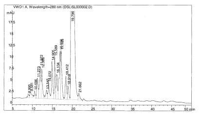
Fig. 5. Sample solution chromatogram (DSL – 19.7 min) in oxidative media
