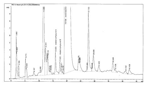
Fig. 2. System suitability chromatogram (contain desloratadine, desloratadine related compound A, desloratadine related compound B)
